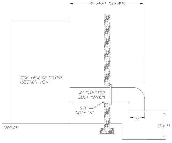
NOTE A: OPENING MUST BE TWO (2) INCHES LARGER THAN THE DUCT (ALL THE WAY AROUND)
